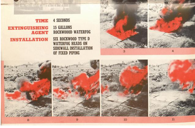
Robot Camera catches vivid split-second pictures of remarkable extinguishing action of Rockwood WATERFOG -- only 4 seconds elapsed between pictures 5 and 10.
